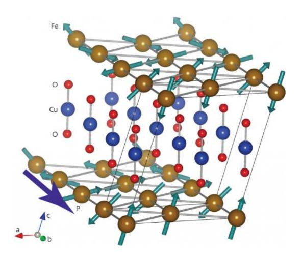
Structure of CuFeO2. The magnetism of the iron atoms (brown, with green arrows showing magnetism) influences the chemical bonds with the other elements (blue: copper, red: oxygen) to create a ferroelectric polarization (purple arrow P). Credit: 2012 The American Physical Society
