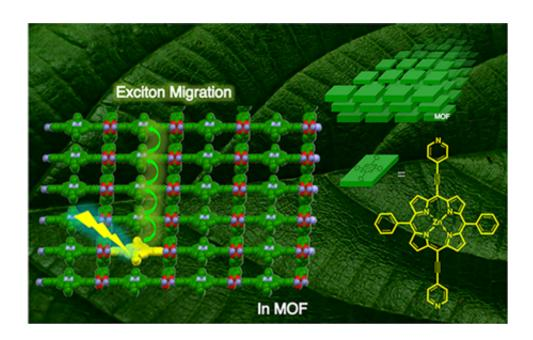
A schematic of directional energy (exciton) migration in the MOF, along with the porphyrin building-blocks of the MOF, is shown.
