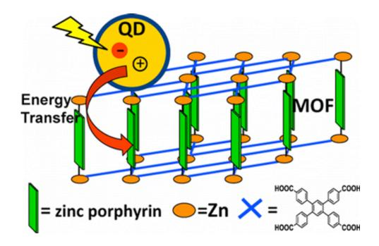
Schematic of QD sensitization and energy transfer to the MOFs; QDs are 5-6 nm and the interporphyrin spacing is about 1 nm.
