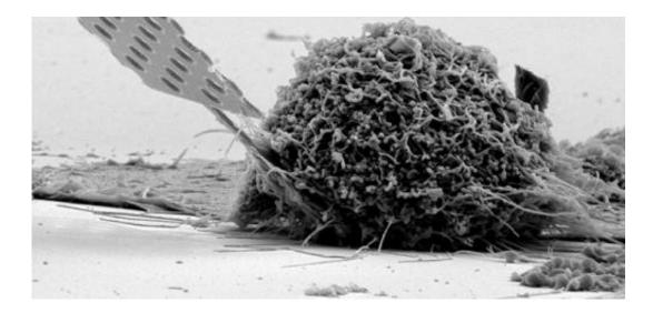
This scanning electron microscope (SEM) image shows a nanobeam probe, including a large part of the handle tip, inserted in a typical cell. Credit: Gary Shambat, Stanford University School of Engineering
