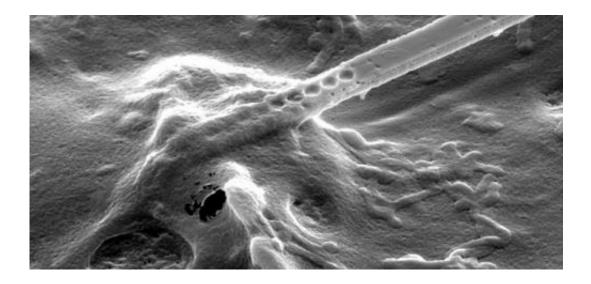
This image shows a photonic nanobeam inserted in a cell. Clearly visible are the etched holes through the beam as well as the sandwich-like layer structure of the beam itself. The beam structure alternates between layers of gallium arsenide and photonic crystal containing the photon-producing quantum dots. Credit: Gary Shambat, Stanford University School of Engineering
