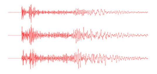
Seismogram of waves picked up from a North Korean nuclear test by a Chinese measuring station. The configuration and magnitude of the waves suggest a blast equal to some 7,000 tons of TNT. Credit: Won-Young Kim, Lamont-Doherty Earth Observatory
