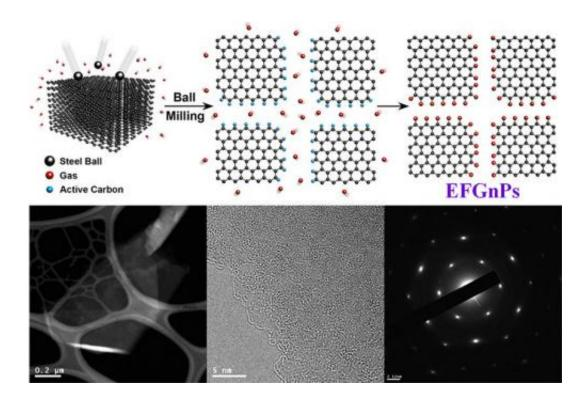
Schematic representation of the mechanochemical reaction between in situ generated active carbon species and reactant gases in a sealed ball-mill crusher. Credit: JACS
