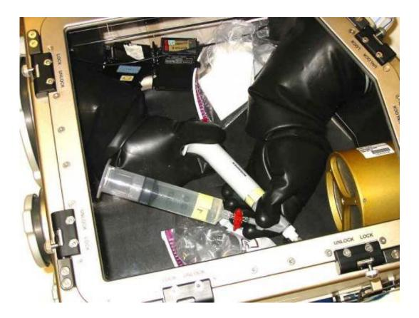
The portable glovebox was used on the International Space Station to perform experiments in a closed environment. This allowed astronauts to work with samples that could endanger the crew if released into the spacecraft's atmosphere.
