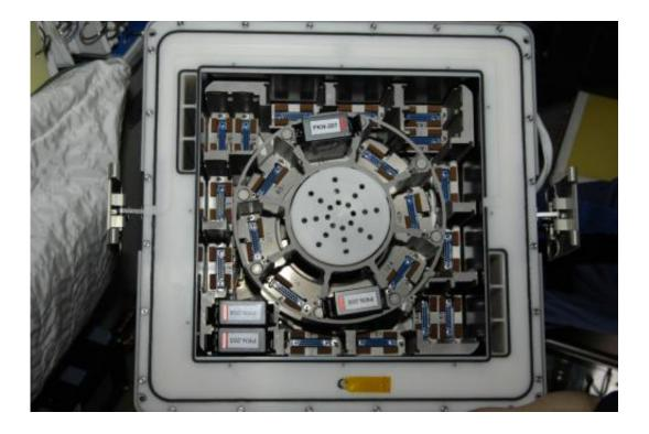
Kubik contains a small centrifuge to simulate Earth-like gravity. In addition, samples placed in Kubik can be kept at controlled temperatures, allowing the box to act as an incubator. Kubik can be configured to perform different experiments on the International Space Station. Credit: ESA–J. Hatton
