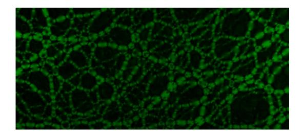
Two-dimensional granular material composed of photo-elastic disks. Regions of high stress appear bright. Researchers can determine contact forces by examining brightness patterns.
