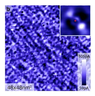
Scanning tunneling microscope image of a 48-nanometer square sample of an iron-based superconductor finds a\n array of dumbbell-shaped "impurities" in the electronic structure, like the sample in the inset, confirming a theoretical prediction. The electronic impurities are associated with cobalt atoms (red cross in the inset). Credit: Davis Lab
