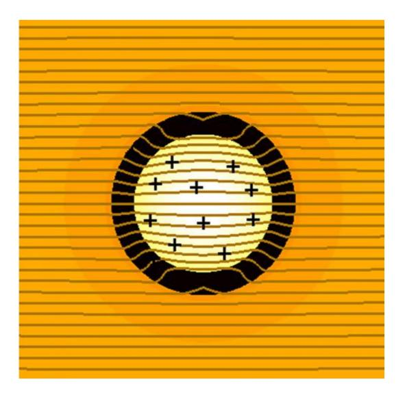
This diagram shows one of the core-shell nanoparticles embedded in a host material, as described in a paper in Advanced Materials. The motion of electrons, as shown by brown lines, is bent in such a way that they appear to be unaffected by the presence of the particle, thus allowing them to pass with little
