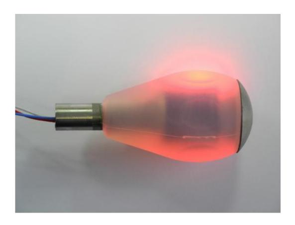
Once the optimal torsional moment is reached, an LED on the inside of the instrument handle lights up. Credit: Fraunhofer IPA
