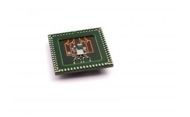
Imec's low-power multi-Gbit 60GHz wireless module integrating a 40nm low-power chip with a 4-antenna array.
