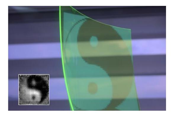
This shows a comparison between the (ground truth) image being focused on the sensor surface and the reconstructed image (inset). Credit: Oliver Bimber, Johannes Kepler University Linz.
