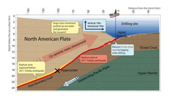
This is a conceptual image of the sub-seafloor structure at the JFAST drilling site. Credit: JAMSTEC/IODP
