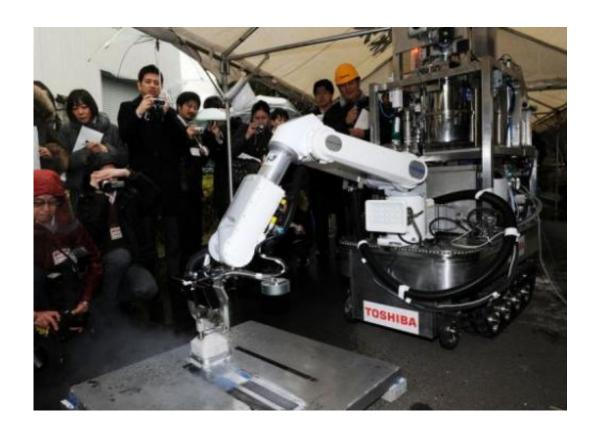
A Toshiba decontamination robot, for work inside a nuclear plant, is used during a demonstration at Toshiba's technical center in Yokohama, suburban Tokyo on February 15, 2013. The crawler robot blasts dry ice particles against contaminated floors or walls and will be used for the decontamination in TEPCO's stricken Fukushima nuclear power plant.
