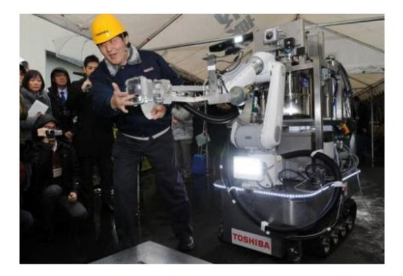
An engineer of Toshiba displays a decontamination robot, for work inside a nuclear plant, during a demonstration at Toshiba's technical center in Yokohama, suburban Tokyo on February 15, 2013. The crawler robot blasts dry ice particles against contaminated floors or walls and will be used for the decontamination in TEPCO's stricken Fukushima nuclear power plant.
