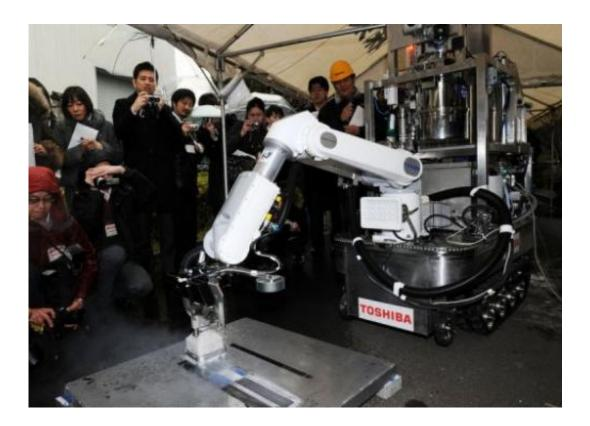
A Toshiba decontamination robot, for work inside a nuclear plant, is used during a demonstration at Toshiba's technical center in Yokohama, suburban Tokyo on February 15, 2013. The crawler robot blasts dry ice particles against contaminated floors or walls and will be used for the decontamination in TEPCO's stricken Fukushima nuclear power plant.
