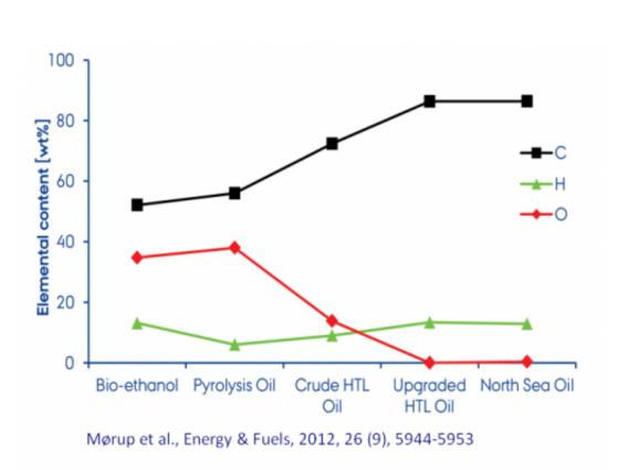
The graphs show the contents of oxygen, hydrogen and carbon in HTL-oil before and after upgrading, compared to other fuel types. Credit: Mørup et al., *Energy* & *Fuels*, 2012, 26 (9), 5944-5953
