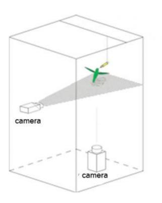
This cartoon shows the experimental setup. High-speed cameras recorded the hovering of hummingbirds in the lab. Credit: Altshuler Lab, UC Riverside.
