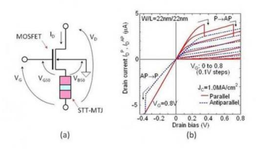
(a) Circuit configuration of PS-MOSFET, in which the STT-MTJ connected to the source of the MOSFET feeds back its voltage drop to the gate, and the degree of negative feedback depends on the resistance state of the STT-MTJ.(b) Simulated output characteristics and current-induced magnetization swiching (CIMS) behavior of the PS-MOSFET.
