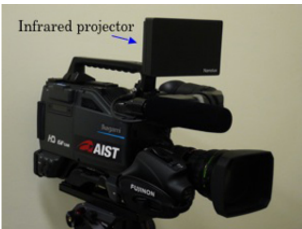
Figure 2 : The newly developed HD infrared color night-vision camera The black rectangular block on top of the camera is the infrared projector.
