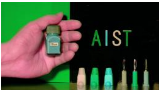
Figure 1 : Example of images of objects taken in darkness by using the newly developed infrared color night-vision camera.
