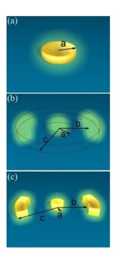
(a) The original metallic object. (b) The metallic object covered by the designed ghost device, metamorphosing scattering feature of the original object. (c) A shrunk metallic object at the original centre with two wing dielectric objects, whose signature is identical to (b). Credit: National University of Singapore
