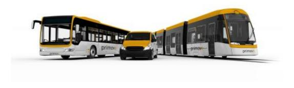
(Phys.org)—Canadian company Bombardier, Inc's rail division based in Berlin Germany, has announced the approval of a test run of an all electric bus recharging system in the city of Mannheim. The power systems are based on the company's PRIMOVE Technology, whereby vehicles are charged inductively while pausing to load and unload passengers. The primary purpose of the test-run is to determine whether such a system is viable in a real-world environment.
