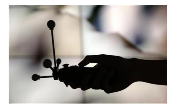
In this photo made Thursday, Jan. 24, 2013, in Chicago is the CAVE2 "wand." The wand and a pair of 3D glasses enables viewers inside CAVE's 72 stereoscopic liquid crystal display panels encircling the viewer 320 degrees, the ability to control movement in the 3D environment that can take you to the bridge of the Starship Enterprise, a flyover of the planet Mars, or through the blood vessels of the brain. (AP Photo/Charles Rex Arbogast)
