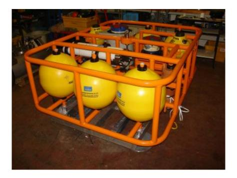
The image shows one of the National Oceanography Centre?s science platforms which will be used to measure turbulence and sediment transport in the nearshore area. Credit: National Oceanography Centre
