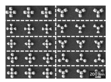
Electron microscope images of two different plasmonic structures that researchers can deconstruct into subunits to determine optical properties. Credit: 2012 American Chemical Society
