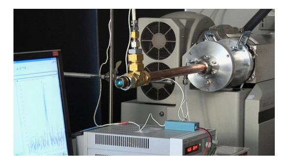
While a commercial-off-the-shelf mass spectrometer is used, the truly unique capability analysis lies in PNNL's ionization chemistry approach developed on the front end of the system.
