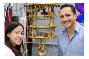
PhD students James Colless and Alice Mahoney preparing a dilution refrigerator for experiments on quantum dots. Temperatures close to absolute zero are required to study the quantum behaviour.
