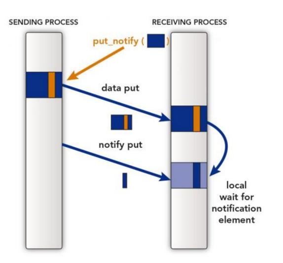
Schematic illustration of push data using a put\_notify call in Global Arrays.
