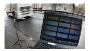
An EPFL doctoral student has designed a microphone-based system that functions as an automatic road traffic sensor. The technology can determine not just how much traffic there is, but also how fast vehicles are going and even their size. It has already sparked an interest in the Swiss towns of Sion and Martigny. Credit: 2013 EPFL
