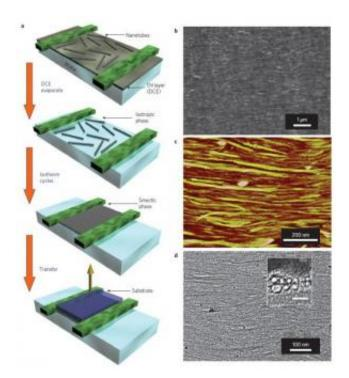
(a) The assembly of a dense, full-coverage nanotube array, and (b) microscopic images of the aligned nanotubes. The study takes carbon nanotubes a step closer to replacing silicon in electronic devices. Image caption: Qing Cao, et al. ©2013 Macmillan Publishers Limited
