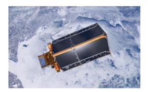
CryoSat's 'roof' is formed from solar panels rigidly fixed to the satellite body, designed to provide adequate power under all orbital conditions for this non-Sun synchronous satellite.
