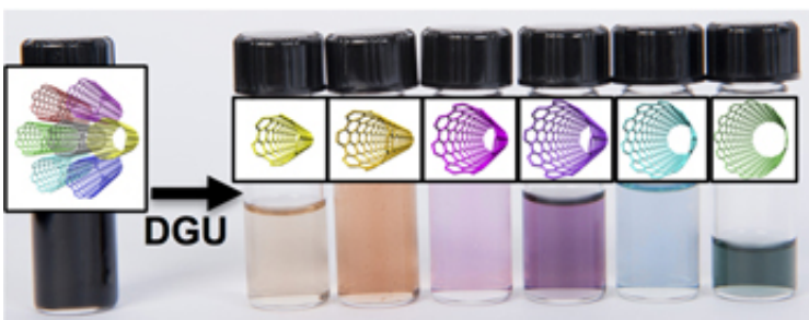
Layers of nanotubes take on different colors after separation via density gradient
