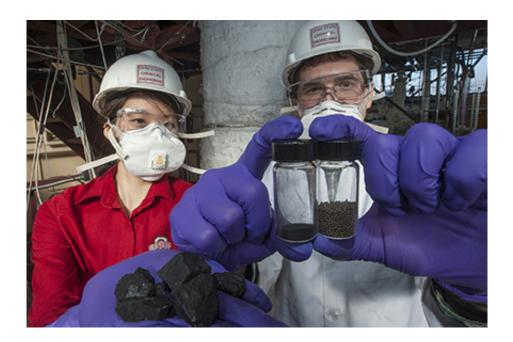
At a research-scale combustion unit at Ohio State University, engineers are testing a clean coal technology that harnesses the energy of coal chemically, without burning it. Here, doctoral student Elena Chung (left) and master's student Samuel ayham (right) display chunks of coal along with pulverized coal (bottle, center) and the iron oxide beads (bottle, right) that enable the chemical reaction. Credit: Photo by Jo McCulty, courtesy of Ohio State University.
