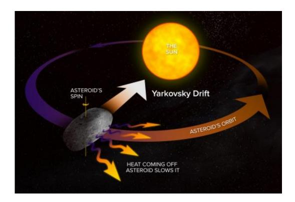
How the Yarkovsky Effect slows an asteroid's orbital motion; opposite rotation direction would speed up the orbital motion. Credit: Alexandra Bolling, NRAO/AUI/NSF
