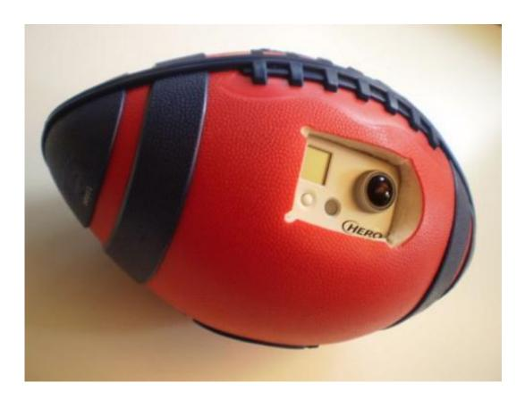
Researchers at Carnegie Mellon University and the University of Electro-Communications placed a small, wireless camera inside a plastic foam football to obtain video while the spiraling ball is in flight. Credit: Carnegie Mellon Robotics Institute
