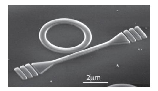
A scanning electron microscope image of one of the quantum photonic devices andrei faraon and his colleagues created. It features a micro-ring resonator coupled to a waveguide. Credit: Faraon/Caltech
