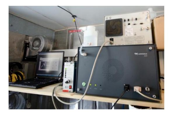
The scanning Particle Size Magnifier, the first instrument for measuring aerosol particles as small as one nm in diameter. Credit: Joonas Vanhanen
