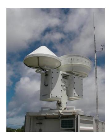
A Scanning ARM Cloud Radar installed at the Manus Island, Papua New Guinea ARM Climate Research Facility. Two radars are mounted on a single scanning pedestal to provide data on the microphysical properties of clouds and precipitation. Credit: ARM
