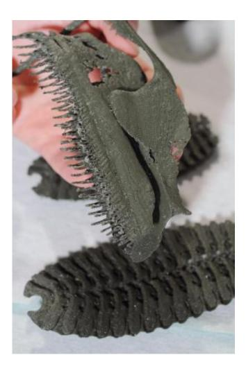
3-D rapid prototypes of an enlarged lamella (in hand) and mineralized tissue within a remora adhesive disk (on table). Researchers at Georgia Tech plan to create an engineered reversible adhesive inspired by the remora that could be used to create pain- and residue-free bandages, attach sensors to objects in aquatic or military reconnaissance environments, replace surgical clamps, and help robots climb. Credit: Gary Meek
