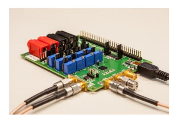
Imec's and Holst Centre's ultra-low power multi-standard 2.4 GHz transceiver compliant with the most common short-range wireless standards (Bluetooth Low Energy, ZigBee, IEEE802.15. 6).
