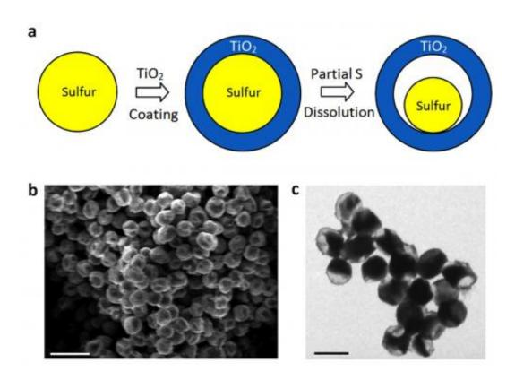
The yolk-shell nanoparticles are made by coating sulfur with a nanoporous layer of hard titanium dioxide, and then using a solvent to dissolve away some of the sulfur while leaving the shell in place. Credit: Zhi Wei She, Stanford
