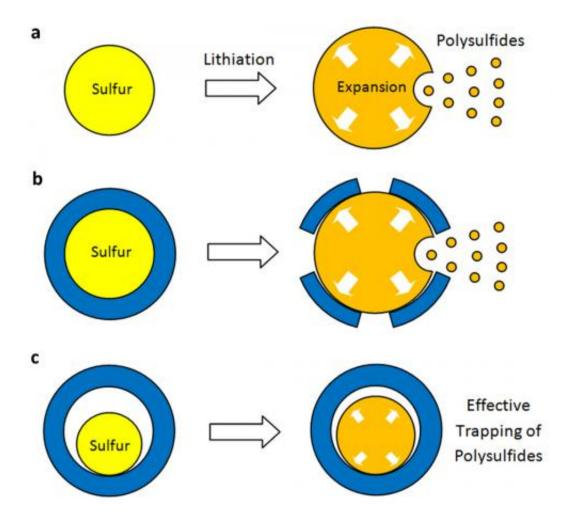
Previous attempts to make sulfur cathodes using bare sulfur or simply coated particles could not prevent the dramatic reduction of energy-storage capacity as the lithium-sulfur intermediate compounds (polysulfides) created during charging broke free and dissolved away.
