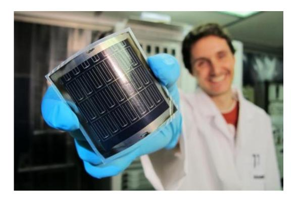
High-efficiency flexible CIGS solar cells on polyimide film were developed at Empa with a novel process. Credit: Empa
