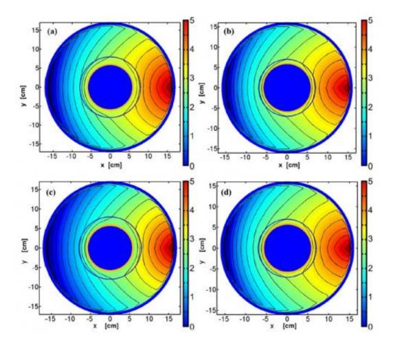
Simulation results of a metallic disk (blue circle) being cloaked by a dc invisibility cloak (thin blue circle surrounding the metallic disk). The color scale represents electric potentials and the thin black lines represent equipotential lines. Outside the cloak, the equipotential lines are almost concentric circles, showing nearly perfect cloaking effects. Credit: Wei Xiang Jiang, et al. ©2013 American Institute of Physics
