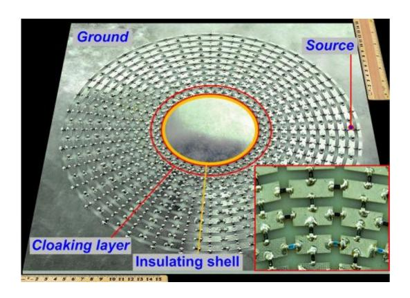
The dc invisibility cloak has a thickness of just one unit cell and can cloak an object nearly perfectly. The inset shows an enlarged view of the cloak's resistor network. Credit: Wei Xiang Jiang, et al. ©2013 American Institute of Physics
