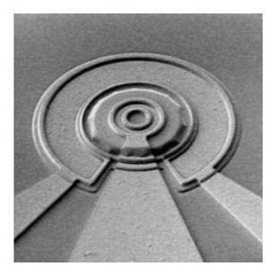
An electron microscope image of the avalanche photodetector developed at A\*STAR. The device measures 30 micrometers in diameter. Credit: 2012 A\*STAR Institute of Microelectronics
