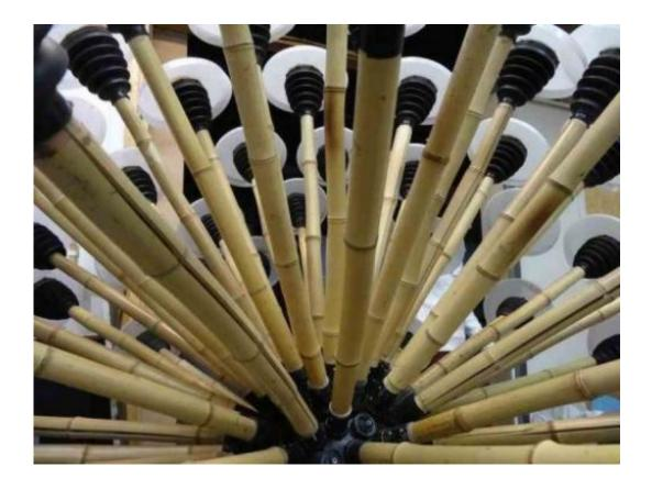
The "mine kafon", a wind-driven gadget to clear anti-personnel mines, could save thousands of lives, its inventors say. With the legs made from bamboo, they are easily replaceable. Once they are blown off it's simply a matter of screwing on others, which means the kafon can be used over and over.
