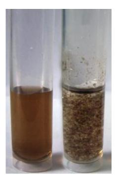
A new method for removing radioactive material from solutions is the result of collaboration between Rice University and Lomonosov Moscow State University. The vial at left holds microscopic particles of graphene oxide in a solution. At right, graphene oxide is added to simulated nuclear waste, which quickly clumps for easy removal. Credit: Anna Yu. Romanchuk/Lomonosov Moscow State University
