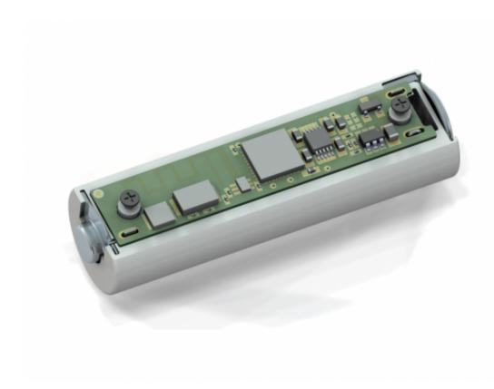
(Phys.org)—An Indiegogo project by Tetherboard drew interest at CES in Las Vegas this week where a novel concept of phone battery was demonstrated. The prototype on show was Tethercell, an adapter which the user can control from a smartphone or tablet, The adapter, powered by a AAA-battery, embeds Bluetooth into a traditional AA battery form.
