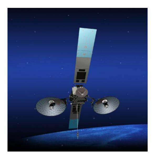
An artist concept of the TDRS-K spacecraft in orbit with its assortment of antennas and a pair of solar arrays to provide electricity. Credit: The Boeing Co.
