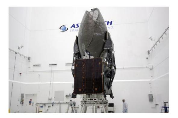
The TDRS-K spacecraft stands inside a processing hangar in Titusville, Fla., awaiting packaging for launch into orbit 22,300 miles above Earth. Credit: NASA/Jim Grossmann
