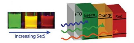
(Left) Photographs under UV light of quantum dots with different ratios of selenium to sulfur, resulting in different colors. (Right) Illustration of the quantum dot layers absorbing different wavelengths of light as the photoanode in a solar cell. Credit: Santra, et al. ©2013 American Chemical Society
