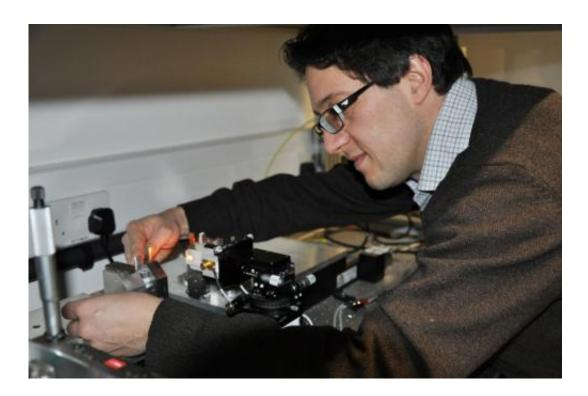
Gilberto mounting a fibre on the nanowire fabrication rig.
