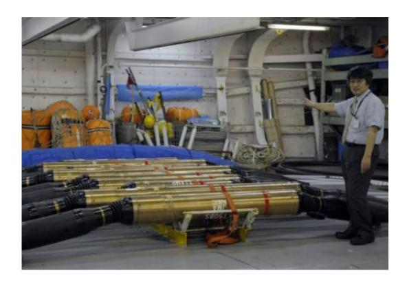
Earthquake and tsunami sensors on the submarine cable construction ship, "Subaru" at Yokohama port on July 3, 2008. A proposed quake early-warning system would use technology already in place in Japan to issue warnings from underground sensors to California.
