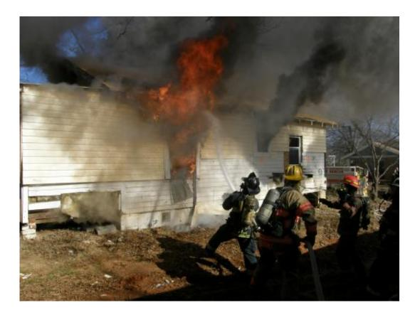
Firefighters in Spartanburg, S.C., battle a "test burn" of an abandoned house in an experiment to demonstrate new techniques for combatting flashover, an extremely dangerous phenomenon in fires. Researchers from NIST, the International Society of Fire Service Instructors, and state and local fire and safety officials participated in the tests the week of Jan. 20, 2013. [Note to editors: Additional photos are available.] Credit: Madrzykowski/NIST
